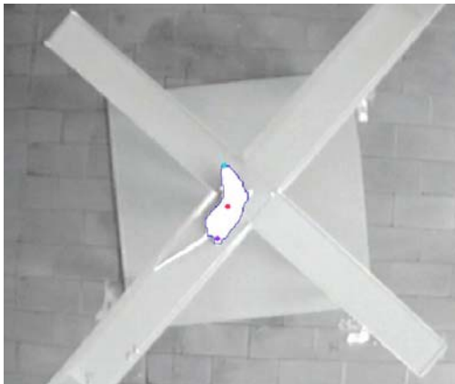
Figure 5.5 An example of good contrast between animal and background, using a white mouse. Furthermore, the transparent walls also help reducing shadows.
