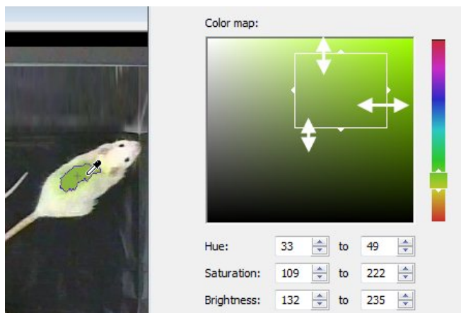
Figure 7.3 The color of the marker after fine-tuning the color settings. Most of the marker is now selected as indicated by the black outline.
