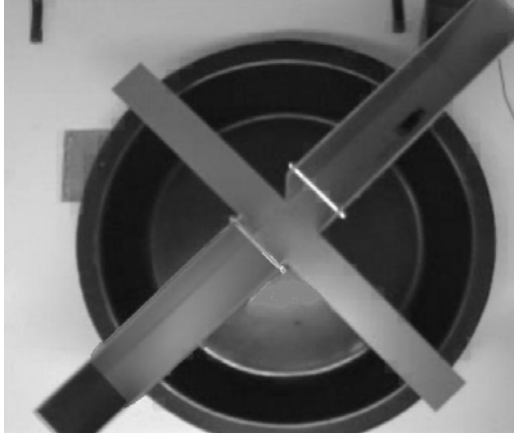
Figure 5.4 In this example, the closed arm at the top-right corner receives little light. This makes detection more difficult when the animal walks in that arm.
