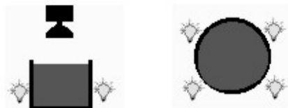
Figure 3.2 Lighting a water maze. Left: view from side, right: view from above.
