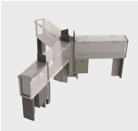
Figure 13.1 A Y-maze setup with automatic doors in each arm.
